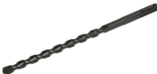
**Features & Benefits** ~ Tungsten carbide tipped with optimized geometry for drilling concrete and stone ~ Vacuum brazed tips for durability ~ Ground flutes designed for optimum debris removal ~ SDS-plus shank ~ Diameter: 25 mm ~ Working length: 350 mm ~ Total length: 450 mm
